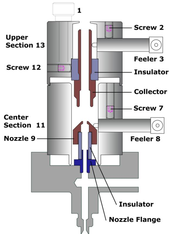
Fig. 31: FID Cross section
