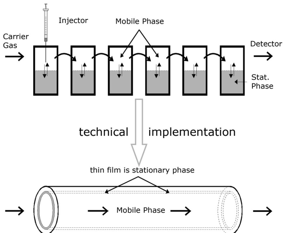
Fig. 20: Distribution in mobile phases
