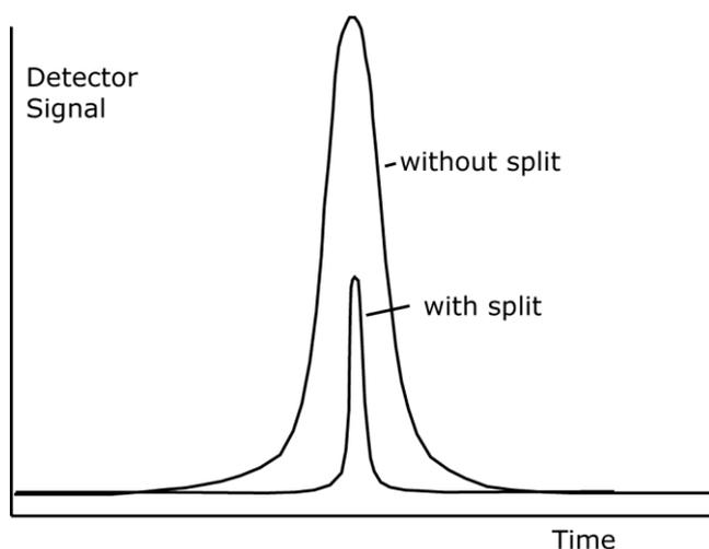
Fig. 24: Concentration profile with and without split
