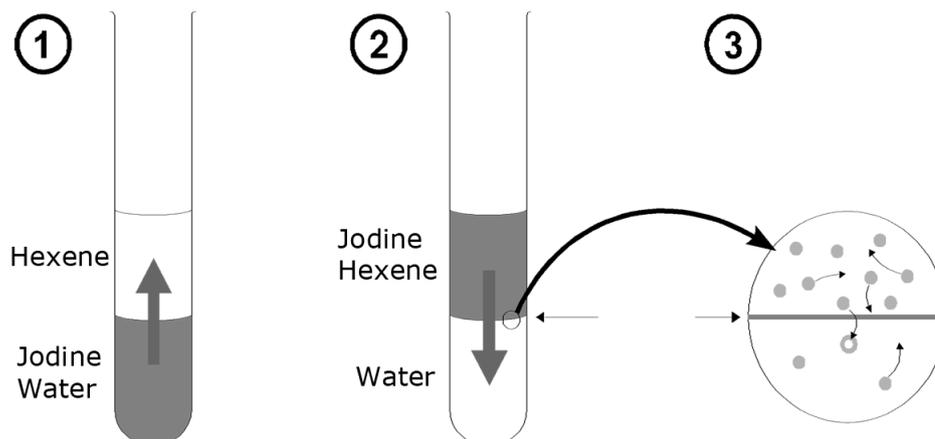
Fig. 19: Distribution between two phases
