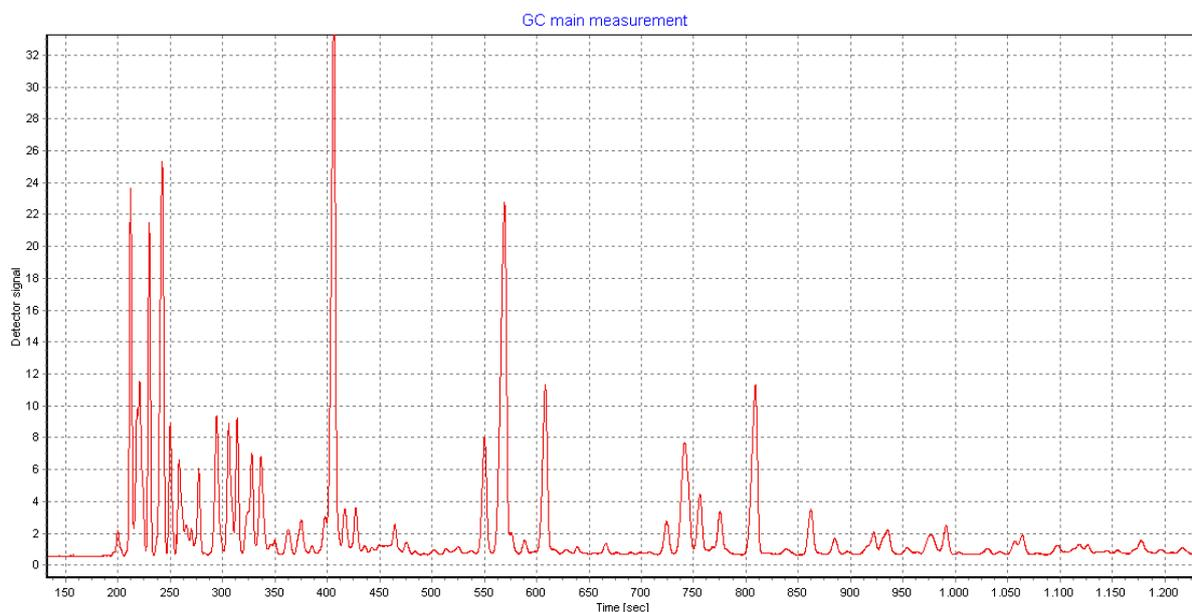
Fig. 12: Chromatogram of supergrade petrol
