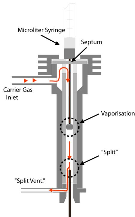
Fig. 23: Injector with split
