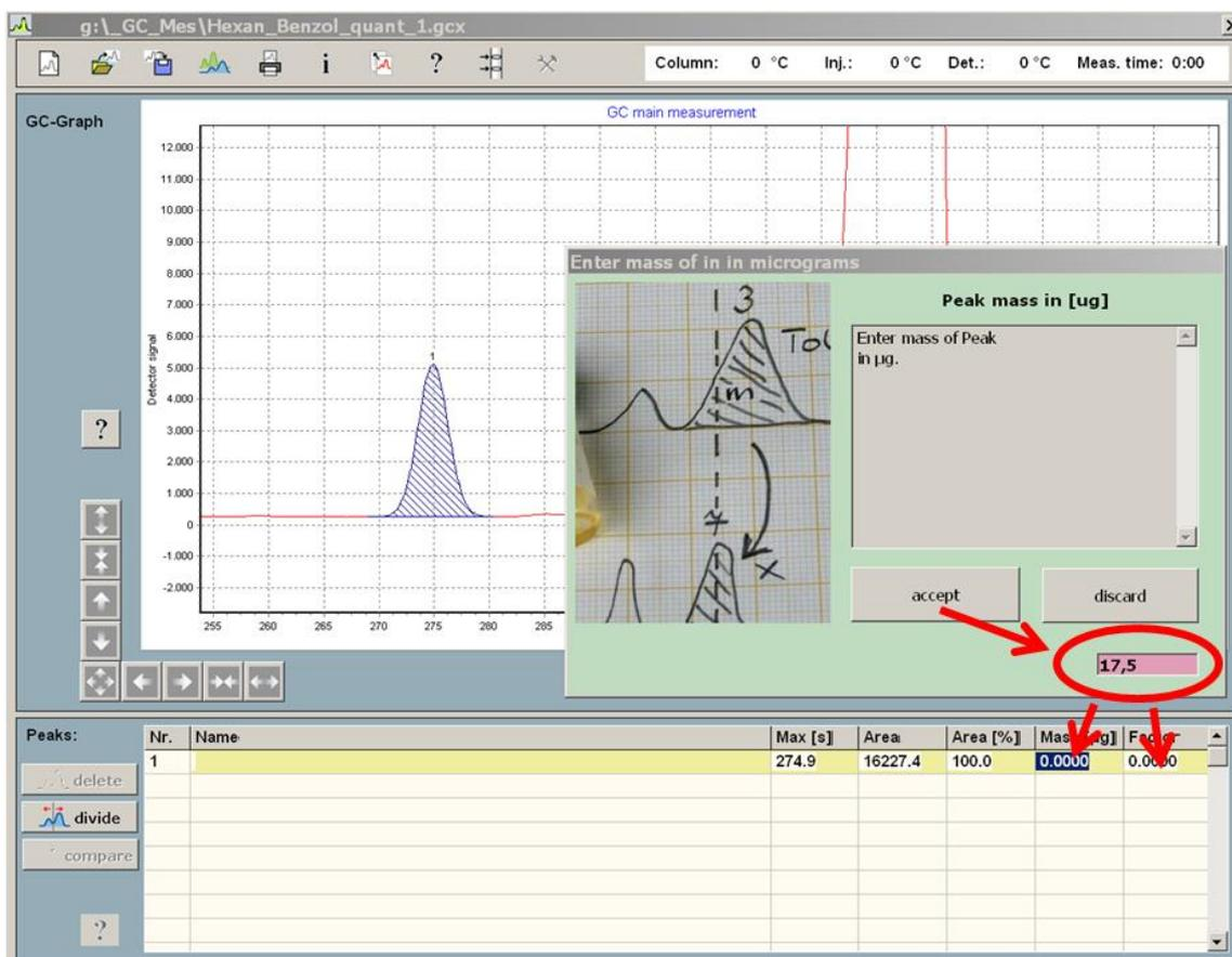
Fig. 16: Reference measurement 'benzene in heptane', entering peak mass
