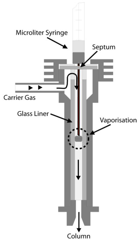
Fig. 22: Injector without split
